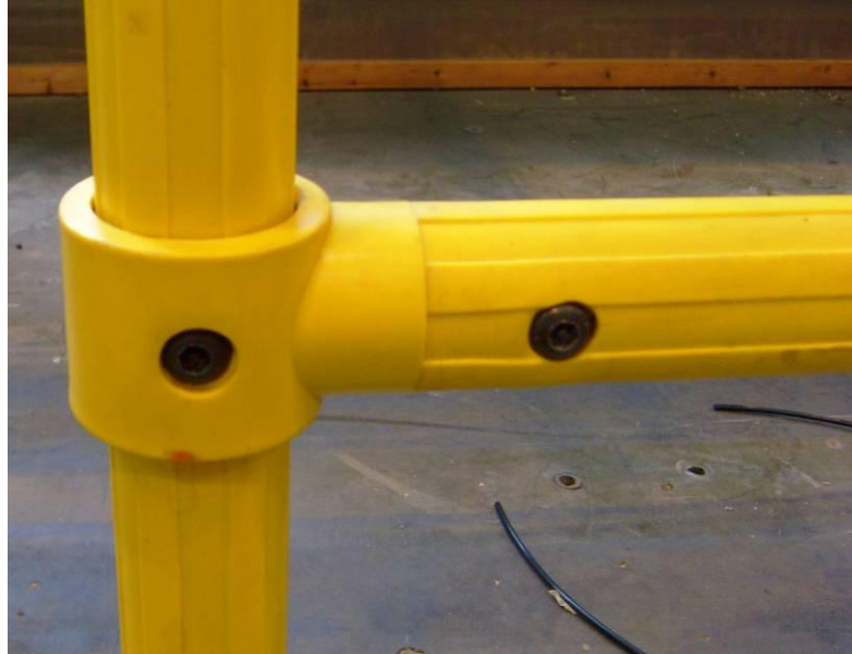
Figure 4: Close-up of knee-rail connection prior to testing
