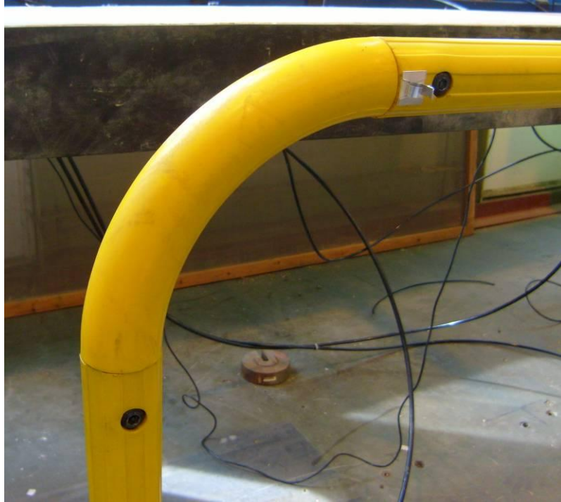
Figure 2: Close-up of top corner connection prior to testing
