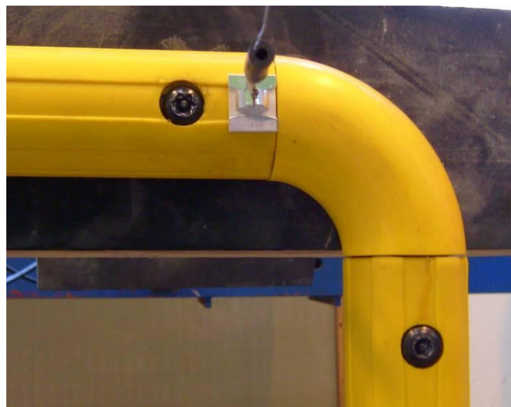
Figure 3: Close-up of top corner connection prior to testing
