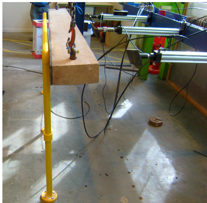
Figure 9: Barrier with load removed showing residual deformation
