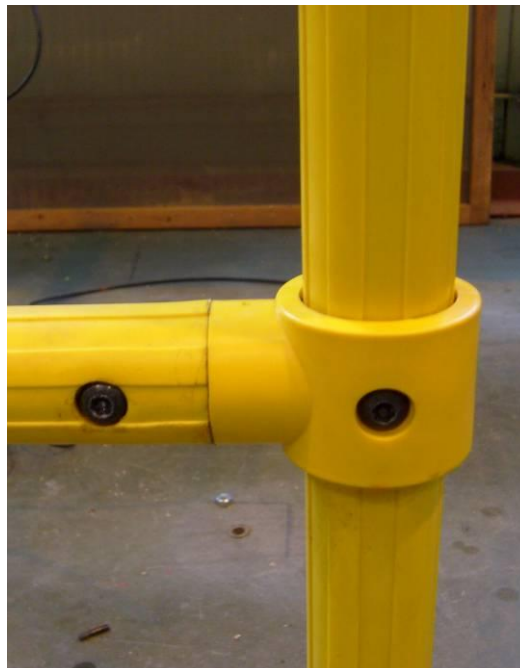
Figure 5: Close-up of knee-rail connection prior to testing
