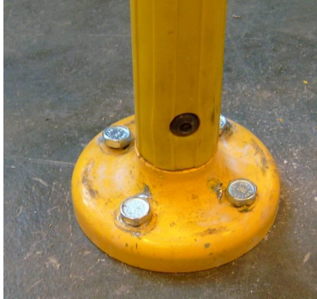
Figure 6: Bolted connection to laboratory floor prior to testing
