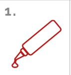
Apply an approx. 6mm bead (this may need to be increased dependant on the substrate conditions) of the high strength gap filling adhesive around the periphery of the underside of the SlipGrip® panels approx. 25mm in from the edges. Then, starting from the bottom left corner come up at an angle (approx. 200mm across) and then down at an angle, to create a 'peak and a trough', repeat this until you reach the end.
