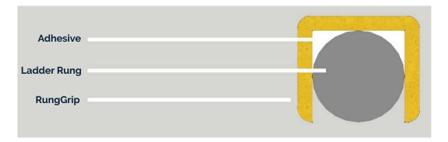
Important: Allow a minimum of 24 hours for the adhesive to cure. Test that the RungGrip Ladder Cover is completely bonded before putting the ladder back into service.
